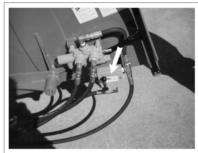
Fig. 22 FLOW CONTROL VALVE
